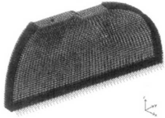
Fig. 5 F.E. model and constraint conditions for the structural mechanics analysis of leaflet (Edwards MIRA bileaflet MHV : thickness= 0.65 mm)
